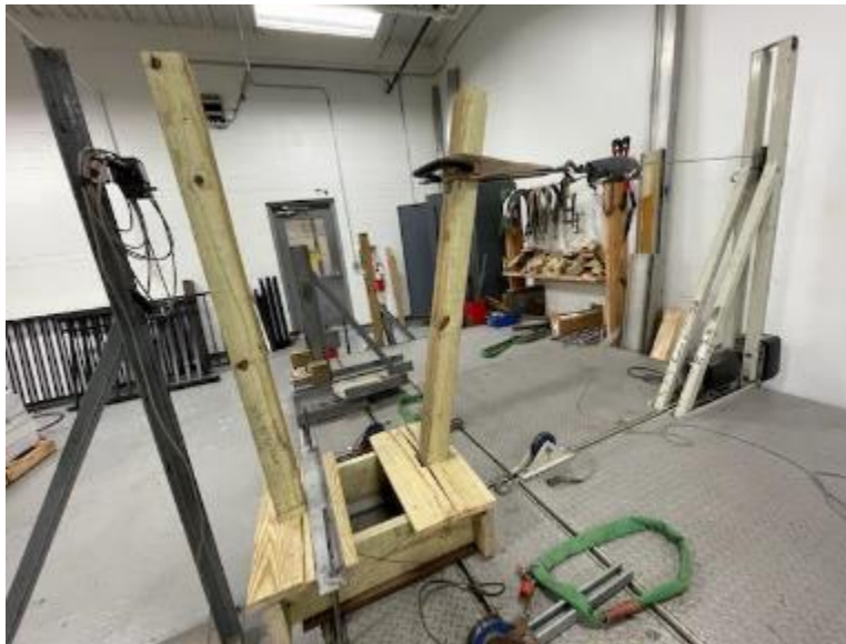
Photo No. 1 Concentrated Load on Top of Single Post
